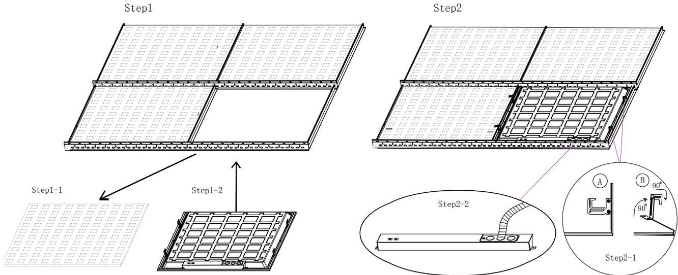
**Step 1:** Make sure of all the power is off before installing. Remove the one ceiling tile that you need to install light fixture on. Then place the light fixture on the T-bar carefully and make sure it is correctly in place and secure.
