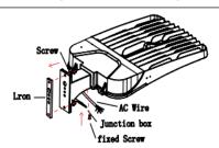
Step 1. Use tools to take screw apart and put installed iron bar away, remove fixed screw and open junction box, then pass the AC wire through it.
