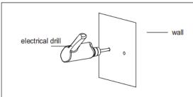
Step 1.Mark the position of the fixing holes with foold lightbracket, then drill the fixing holes.
