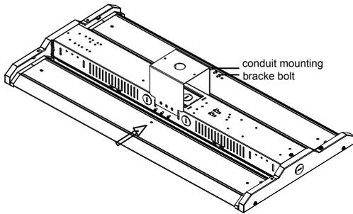
2. Lock the conduit with flat washer+ spring washer+ nut on the mounting bracket.
