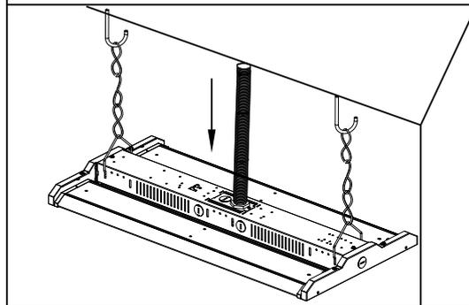
7. Adjust the fixture lighting angle to the direction needed (Shown as below fig).
