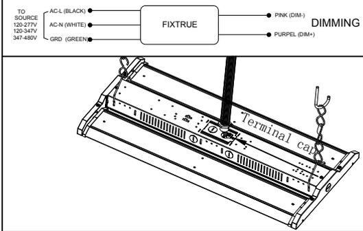
3. Hook up the chain on the ceiling anchor.
