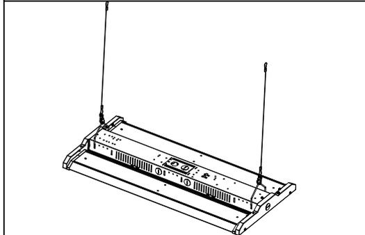
3. Hook the other end of Lifting rope to the ceiling anchor.
