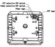
3.After finish the requires power and CCT adjustment, Tighten the M25 cap clockwise by slot type screwdriver.
