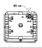
2.According to the tags,customer can select the corresponding power and CCT dip switch, dial to the required power(40w/60w/80w) and CCT(35K/40K/50K).
