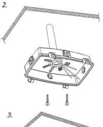
2. Cut off the power supply, rotate the back cover into the 3/4 thread pipe, put the input wire through the hole and make necessary waterproof protection.
