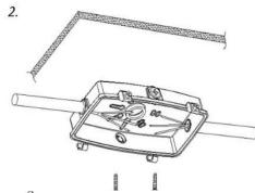
2. Cut off the power supply, rotate the back cover into the 3/4 thread pipe, put the input wire through the hole and make necessary waterproof protection.
