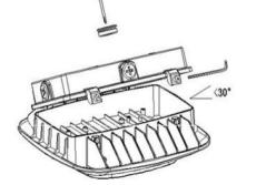
1. Remove the 3/4 plug with a cross screwdriver and take it out. After loosening the screw with an Allen wrench, keep the back cover opened (the angle is less than 30  $^{\circ}$ ) and take it out after turning over.
