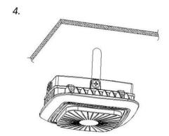
4. Turn over and close the lamp body, lock the screw with the Allen wrench, and install it.
