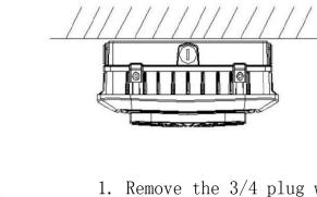
1. Remove the 3/4 plug with a cross screwdriver and take it out. After loosening the screw with an Allen wrench, keep the back cover opened ( the angle is less than 30  $^\circ$  ) and
