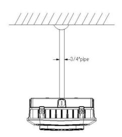
1. Remove the 3/4 plug with a cross screwdriver and take it out. After loosening the screw with an Allen wrench, keep the back cover opened (the angle is less than 30  $^{\circ}$  ) and take it out after turning over.
