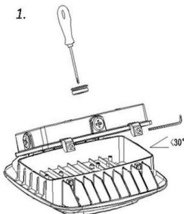
1. Remove the 3/4 plug with a cross screwdriver and take it out. After loosening the screw with an Allen wrench, keep the back cover opened ( the angle is less than  $30^\circ$  ) and take it out after turning over.
