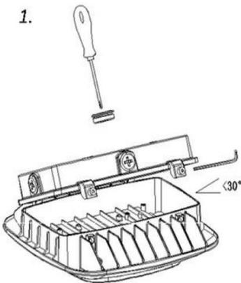
1. Remove the 3/4 plug with a cross screwdriver and take it out. After loosening the screw with an Allen wrench, keep the back cover opened ( the angle is less than  $30^{\circ}$  ) and
