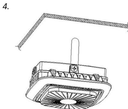
4. Turn over and close the lamp body, lock the screw with the Allen wrench, and install it.
