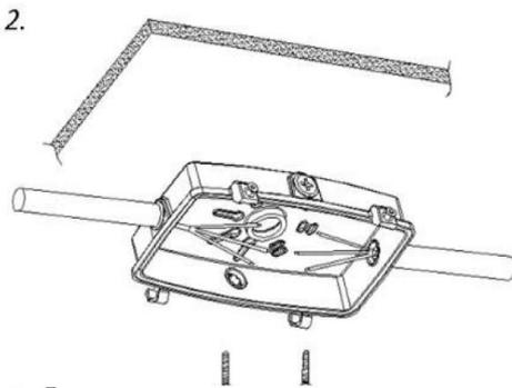
2. Cut off the power supply, rotate the back cover into the 3/4 thread pipe, put the input wire through the hole and make necessary waterproof protection.
