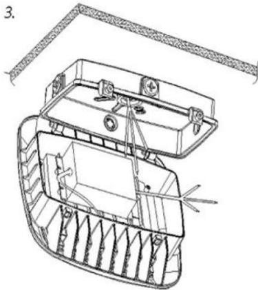
3. Hang the lamp on the back cover at less than 30 degrees, let the lamp fall naturally, and then connect Live line, Neutral line and Earth line.
