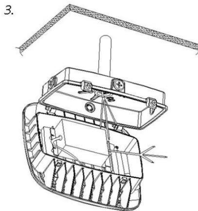
3. Hang the lamp on the back cover at less than 30 degrees, let the lamp fall naturally, and then connect Live line, Neutral line and Earth line.
