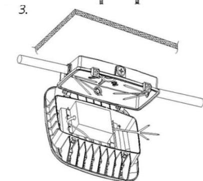
3. Hang the lamp on the back cover at less than 30 degrees, let the lamp fall naturally, and then connect Live line, Neutral line and Earth line.
