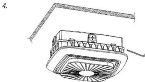
4. Turn over and close the lamp body, lock the screw with the Allen wrench, and install it.
