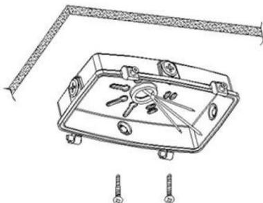
2. Cut off the power supply, use tools to knock out the corresponding installation holes of the back cover, put the input wire through the hole, fix the back cover on the ceiling with screws, and make necessary waterproof protection.
