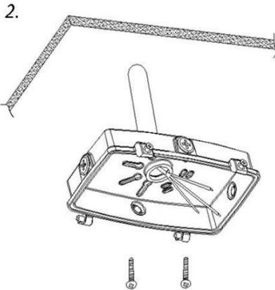
2. Cut off the power supply, rotate the back cover into the 3/4 thread pipe, put the input wire through the hole and make necessary waterproof protection.
