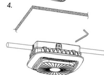
4. Turn over and close the lamp body, lock the screw with the Allen wrench, and install it.
