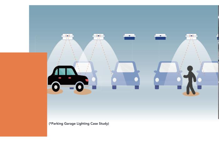
The professional lighting design team not only provides the lighting control system, but also provides lighting design schemes for free. This is a complete set of 400 series Vapor Tight Light with motion sensor control solution and for a whole area to eliminate scattered dark areas that existed while walking or driving through the garage.
