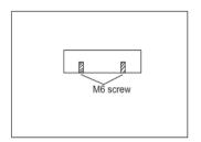
Mark the bracket install hole's position on the wall. The distance is 280+/-20 mm for 2fT, 830+/-20mm for 4fT,1110+/-20mm for 5fT
