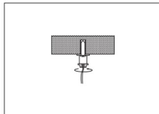
**3** Screw the suspension cable on the ceiling
