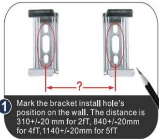
**1** Mark the bracket install hole's position on the wall. The distance is 310+/-20 mm for 2FT, 840+/-20mm for 4FT, 1140+/-20mm for 5FT
