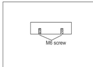
**2** Mark the bracket install hole's position on the wall. The distance is 280+/-20 mm for 2FT, 830+/-20mm for 4FT, 1110+/-20mm for 5FT
