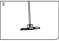
3.Lock the plate by screw nut.
