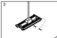
3.Installed fixed clamp, aim at holes.
