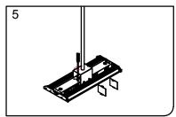
5.After the power cord is correctly connected, reinstall the access plate.
