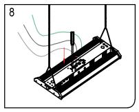
8.After the power cord is correctly connected, reinstall the access plate.
