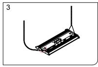
3.Install the hook into the hole, rotary hook up.
