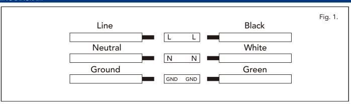
Universal voltage driver permits operation at 120-277V, 50/60 Hz. Follow wiring directions as in Fig. 1.
