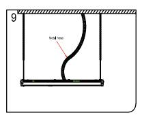
9. Wrap wires with metal material.
