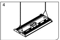
3.Connect the chain to the installation location, and adjust the lamp high, level and balance.
