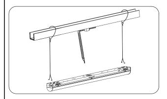
4. Connect the AC wires.
