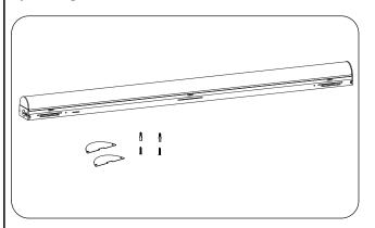
2. Fix the baffle onto the back of the fixture.
