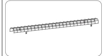
2. Fasten the chips by screws into the prepunched holes of the fixture body.
