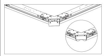
2. Secure the interconnection bracket with screws.
