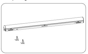
2. Attach V-hooks to the cable.
