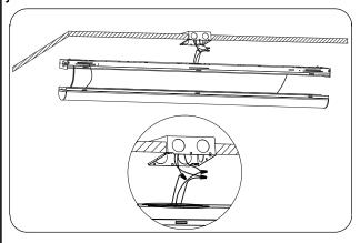
6. Assemble the module board upwards. The installation is complete.
